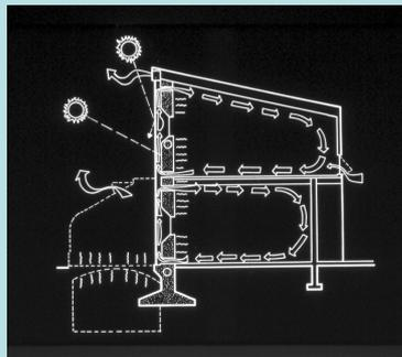
The Trombe wall delays the arrival of solar heat, while the sunspace and direct gain openings allow morning warm-up.
