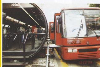
14. Bus with platforms extended to tubular passenger loading point: Wright Collection
